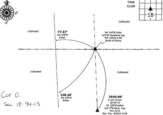
Center of Section 18-94-13 Fd. 8" X 8" Granite Stone, Set 5/8"Ø rebar w/2"Ø aluminum cap PLS 15525 0.50' North
