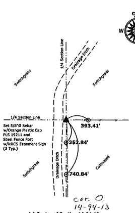
1.) Center of Section 14-94-13 Set 5/8"Ø rebar w/2"Ø aluminum cap PLS 19211
