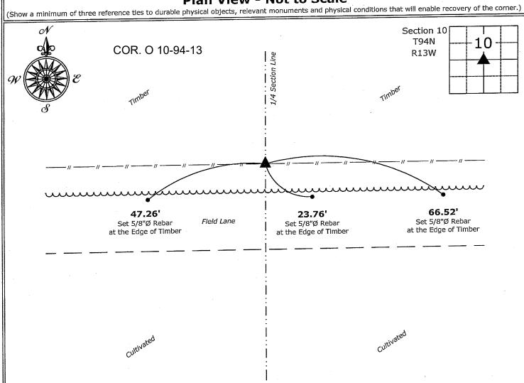
Center of Section 10-94-13 Set 5/8"Ø Rebar w/2"Ø Aluminum Cap PLS 19211
