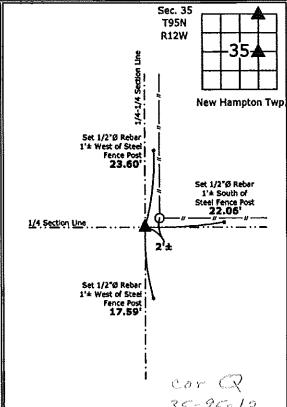
1.) Northeast Corner NW 1/4-NE 1/4 Section 35-95-12 Set Survey Mark Nall w/Stainless Steel Washer PLS 15525
