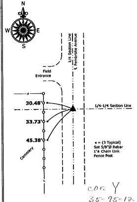
1.) Southwest Corner NW 1/4-NE 1/4 Section 35-95-12 Set 5/8°Ø rebar w/2°Ø aluminum cap PLS 15525
