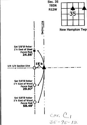
2.) Southeast Corner NE 1/4-NE 1/4 Section 35-95-12 Set 5/8"Ø rebar w/2"Ø aluminum cap PLS 15525
