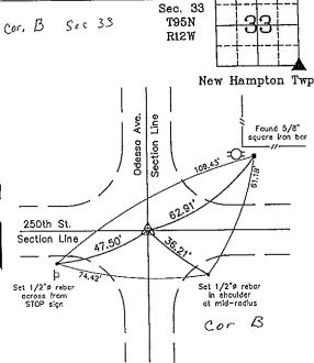
SE Corner Section 33 T95N R12W Found 5/8" square Iron bar, 1—% deep. Set 1/2"ø rebar w/2"ø aluminum cap PLS 16961 over iron bar.
