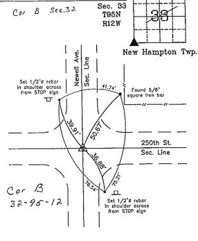
SW Corner Section 33 T95N R12W Found 5/8" square iron bar, 2-½' deep. Set 1/2"ø rebar w/2"ø aluminum cap PLS 16961 over bar.
