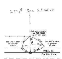
N 1/4 Corner Section 28 T95N R12W Set 1/2"ø rebar w/2"ø aluminum cap PLS 16961
