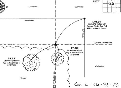
Northeast Corner SW 1/4-NE 1/4 of Section 26-95-12 Set 5/8"Ø Rebar with Aluminum Cap PLS 19211
