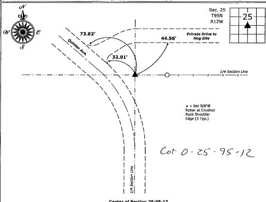
Center of Section 25-95-12 Set 5/8"Ø Rebar with Aluminum Cap PLS 19211
