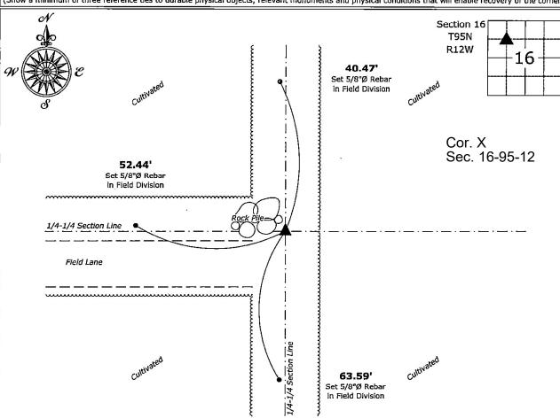
Southeast Corner of the NW 1/4 - NW 1/4 of Section 16-95-12 Set 5/8"Ø Rebar w/2"Ø Aluminum Cap PLS 19211
