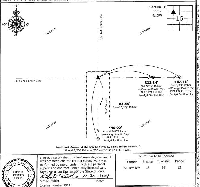
Southeast Corner of the NW 1/4-NW 1/4 of Section 16-95-12 Found 5/8"Ø Rebar w/2"Ø Aluminum Cap PLS 19211
