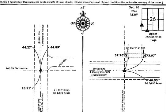
1.) Southwest Corner NW 1/4-SW 1/4 Section 26-97-12 Set 5/8"Ø rebar w/2"Ø aluminum cap PLS 19211
