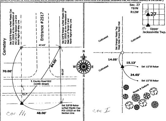
1.) SW Corner SE 1/4-SW 1/4 Section 27-97-12 Set 5/8"Ø rebar w/2"Ø aluminum cap PLS 15525
