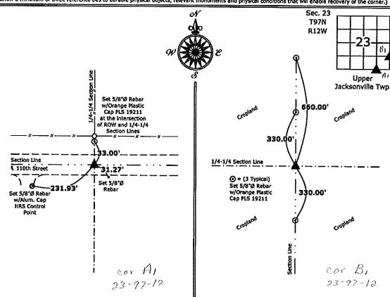
1.) Southwest Corner SE 1/4-SE 1/4 Section 23-97-12 Set 5/8"Ø rebar w/2"Ø aluminum cap PLS 19211
