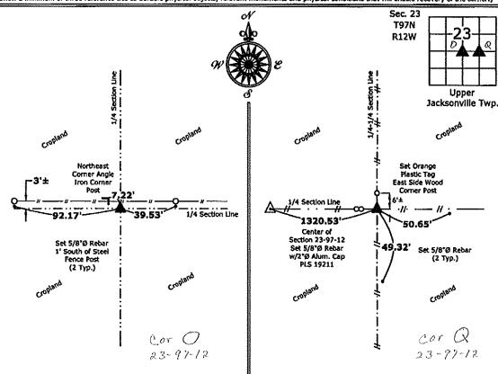
1.) Center of Section 23-97-12 Set 5/8"Ø rebar w/2"Ø aluminum cap PLS 19211 2.) Northwest Corner NE 1/4-SE 1/4 Section 23-97-12 Set 5/8"Ø rebar w/2"Ø aluminum cap PLS 19211
