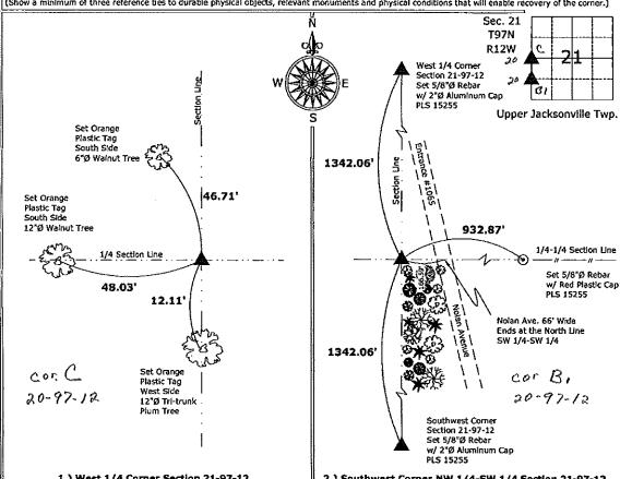
1.) West 1/4 Corner Section 21-97-12 Set 5/8"Ø Rebar w/ 2" Aluminum Cap PLS 15255 2.) Southwest Corner NW 1/4-SW 1/4 Section 21-97-12 Set 5/8\*Ø Rebar w/ 2\*Ø Aluminum Cap PLS 15255
