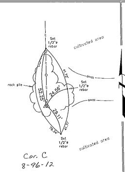
W 1/4 Corner Section 9 T96N R12W Found 1/2"ø rebar w/orange plastic cop LS 7060
