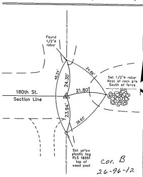
NE Corner Section 35 T96N R12W Set 1/2"ø rebar w/2"ø aluminum cap PLS 16961
