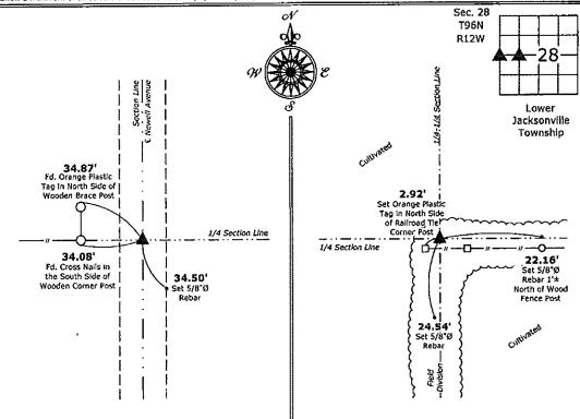
1.) West 1/4 Corner Section 28-96-12 Fd. 5/8"Ø rebar 2.) Northwest Corner NE 1/4 - SW 1/4 Section 28-96-12 Set 5/8\*Ø rebar w/2\*Ø aluminum cap PLS 19211
