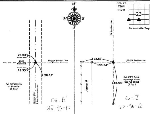
1.) Southwest Corner NW 1/4-SW 1/4 Section 23-96-12 Set 5/8"Ø rebar w/2"Ø aluminum cap PLS 19211
