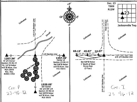
1.) Northwest Corner NE 1/4-SW 1/4 Section 23-96-12 Set 5/8"Ø rebar w/2"Ø aluminum cap PLS 19211 2.) Southwest Corner NE 1/4-SW 1/4 Section 23-96-12 Set 5/8"Ø rebar w/2"Ø aluminum cap PLS 19211
