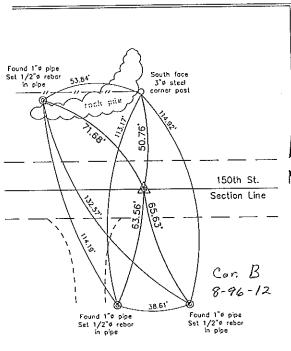
SW Corner Section 9 T96N R12W Found 3/4"ø iron pin, 18" deep. Ralsed with 1/2"ø rebor w/2"ø aluminum cap PLS 16961
