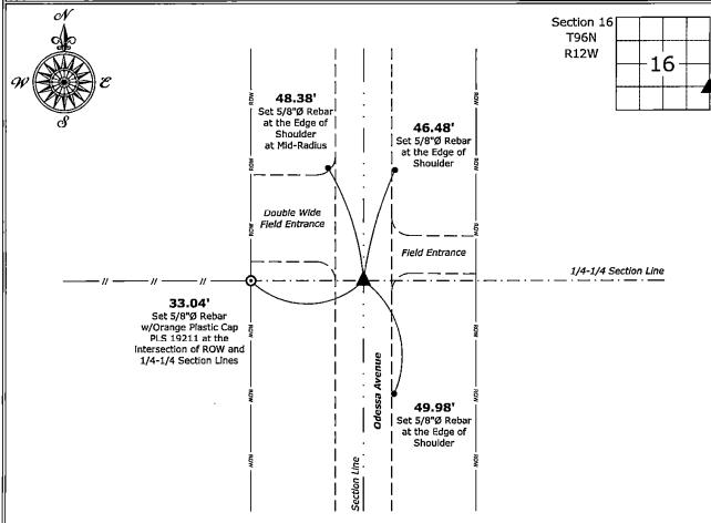
Northeast Corner of the SE 1/4 - SE 1/4 of Section 16-96-12 Set 5/8"Ø Rebar w/2"Ø Aluminum Cap PLS 19211
