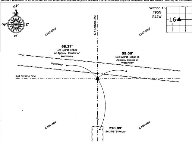
Center of Section 16-96-12 Set 5/8"Ø Rebar w/2"Ø Aluminum Cap PLS 19211 (Buried 18" Deep)
