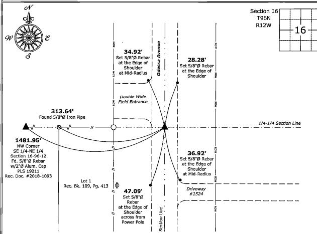
Northeast Corner of the SE 1/4 - NE 1/4 of Section 16-96-12 Set 5/8"Ø Rebar w/2"Ø Aluminum Cap PLS 19211
