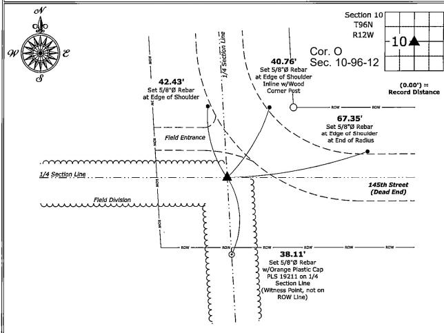
Center of Section 10-96-12 Found 1/2"Ø Rebar
