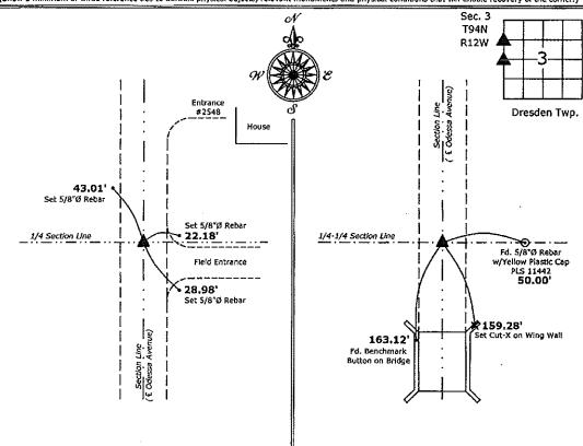
1.) West 1/4 Corner Section 3-94-12 Fd. 1/2"Ø rebar w/1.5"Ø aluminum cap PLS 11442 2.) Southwest Corner NW 1/4-NW 1/4 Section 3-94-12 Fd. 1/2\*Ø rebar w/1.5\*Ø aluminum cap PLS 11442
