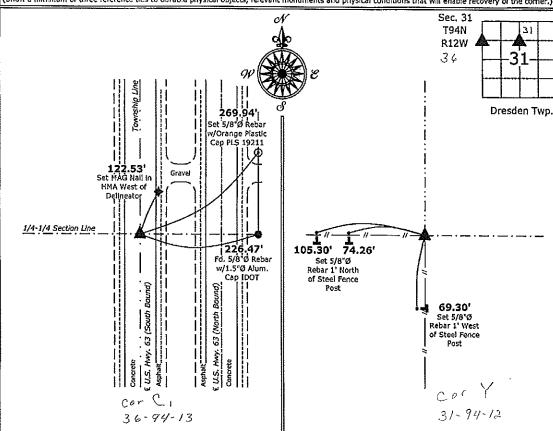
1.) Southwest Corner NW 1/4-NW-1/4 Section 31-94-12 Set Survey Mark Nail w/Stainless Steel Washer PLS 19211
