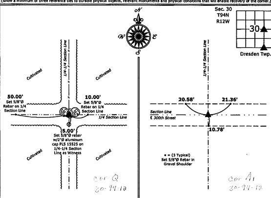
1.) Northeast Corner NW 1/4-SE 1/4 Section 30-94-12 Set 5/8\*Ø rebar w/2\*Ø aluminum cap PLS 15525 as Witness
