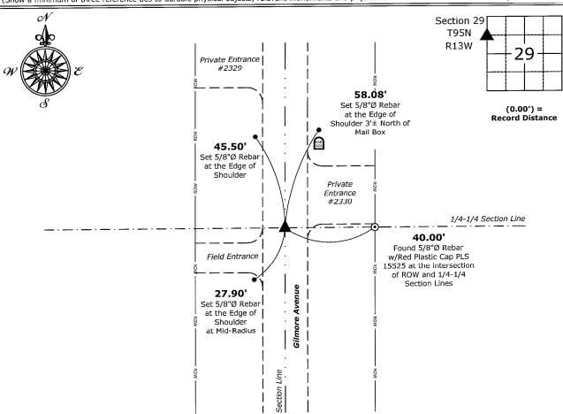
Northwest Corner of the SW 1/4 - NW 1/4 of Section 29-95-13 Found 5/8"Ø Rebar w/2"Ø Aluminum Cap PLS 19211
