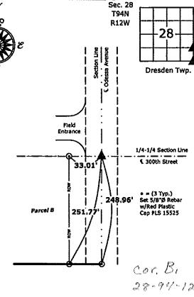
2.) Northeast Corner SE 1/4-SE 1/4 Section 28-94-12 Set 5/8\*Ø rebar w/2\*Ø aluminum cap PLS 15525
