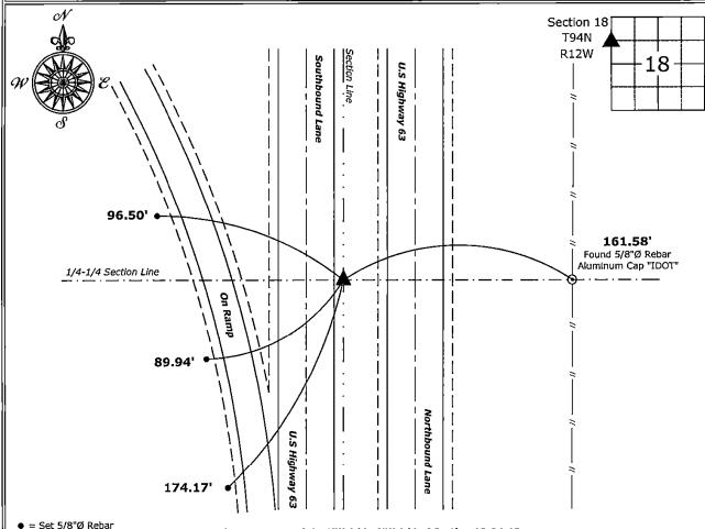
= Set 5/8"Ø Rebar1' North of Delineator Post(3 Typical)
