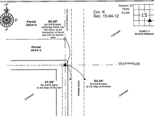
Southeast Corner of the NW 1/4 - SE 1/4 of Section 15-94-12 Set 5/8"Ø Rebar w/2"Ø Aluminum Cap PLS 19211
