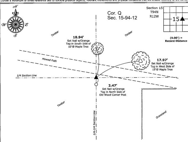
Northeast Corner of the NW 1/4 - SE 1/4 of Section 15-94-12 Set 5/8"Ø Rebar w/2"Ø Aluminum Cap PLS 19211
