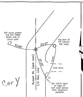
SW Corner NW 1/4 - NE 1/4 Section 13 T94N R12W Set MAG nail w/stainless steel washer PLS 16961
