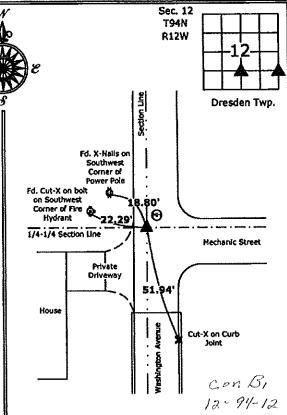
1.) Southwest Corner NW 1/4-SE 1/4 Section 12-94-12 Set 5/8"Ø rebar w/2"Ø aluminum cap PLS 19211 2.) Southeast Corner NE 1/4-SE 1/4 Section 12-94-12 Found MAG nail w/stainless steel washer PLS 11442
