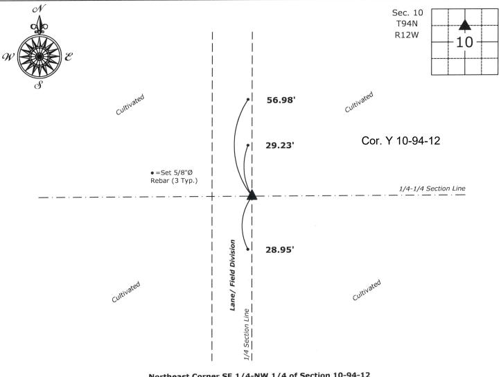
Northeast Corner SE 1/4-NW 1/4 of Section 10-94-12 Set 5/8"Ø Rebar with Aluminum Cap PLS 19211
