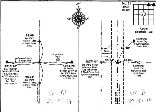
1.) Northwest Corner NE 1/4-NE 1/4 Section 32-97-14 Set 5/8"Ø rebar w/2"Ø aluminum cap PLS 19211
