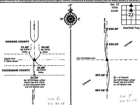
1.) North 1/4 Corner Section 22-97-14 Fd. 2"Ø Gas Pipe 2.) Southwest Corner NW 1/4-NE 1/4 Section 22-97-14 Set 5/8\*Ø rebar w/2\*Ø aluminum cap PLS 15525
