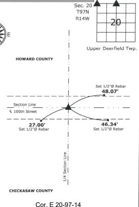
1.) NW Corner Section 20-97-14 Set 5/8"Ø rebar w/2"Ø aluminum cap PLS 19211 2.) North 1/4 Corner Section 20-97-14 Found 5/8"Ø rebar
