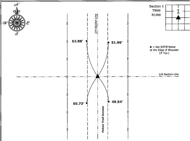
Center of Section 1-96-14 Set 5/8"Ø Rebar w/2"Ø Aluminum Cap PLS 19211
