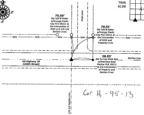
Southwest Corner SE 1/4 - SW 1/4 Section 4-95-13 Set Survey Mark Nail w/Stainless Steel Washer PLS 19211
