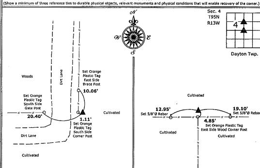
1.) NE Corner SE 1/4-NW 1/4 Section 4-95-13 Set 5/8"Ø rebar w/2"Ø aluminum cap PLS 1552S
