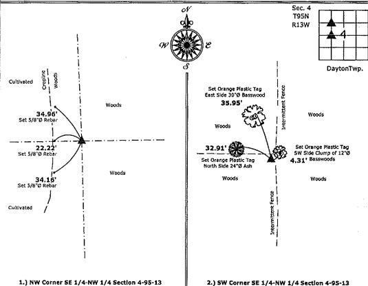
1.) NW Corner SE 1/4-NW 1/4 Section 4-95-13 Set 5/8"Ø rebar w/2"Ø aluminum cap PLS 15525
