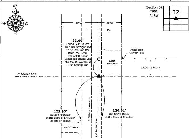
Center of Section 32-95-13 Set 5/8"Ø Rebar w/2"Ø Aluminum Cap PLS 19211
