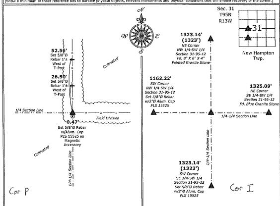
1.) Northeast Corner NW 1/4-SW 1/4 Section 31-95-13 Fd. 8" X 6" X 4" Pointed Granite Stone
