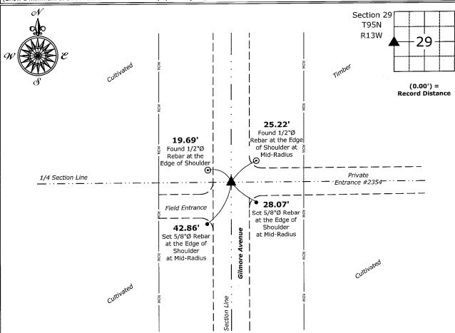
West 1/4 Corner of Section 29-95-13 Found 5/8"Ø Rebar w/2"Ø Aluminum Cap PLS 15525
