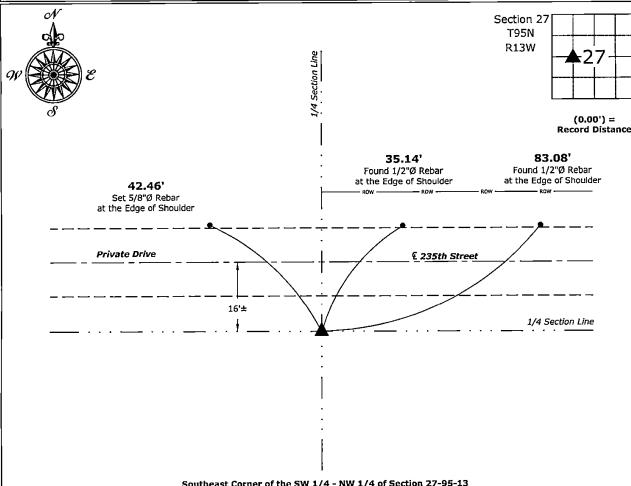
Southeast Corner of the SW 1/4 - NW 1/4 of Section 27-95-13 Found bent 5/8"Ø Rebar, straightened, lowered and placed Aluminum Cap PLS 19211 on top
