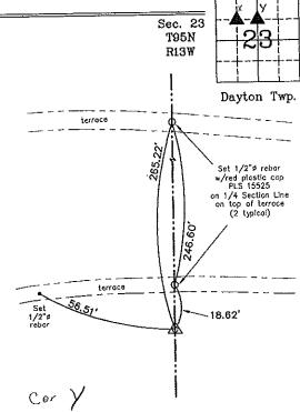
SE Corner NE 1/4 - NW 1/4 Section 23 T95N R13W Set 1/2\*ø rebar w/2\*ø aluminum cap PLS 15525
