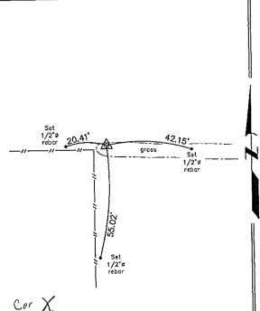
SW Corner NE 1/4 - NW 1/4 Section 23 T95N R13W Set 1/2\*¢ rebar w/2\*¢ aluminum cap PLS 15525
